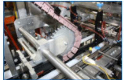
**Servo Driven Top Squaring Chain ensures sleeve closures are positive and consistent. In addition, a high-speed rotary feeder allows for speeds over 200 ppm.**
