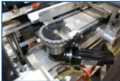
**All major actuated components on the HD-CMS are servo driven. This allows for a plethora of benefits including fast changeover, smooth operation and easy set up.**
