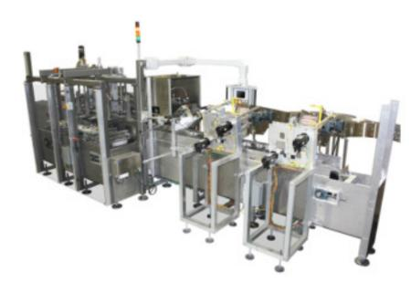
The new MK-BIB Bag in Box Autoload Cartoner is described as a robust packaging system capable of speeds of up to 150 cpm. It can easily changeover with many single point adjustments. Upgrades to fully servo automatic changeover are available which further reduce changeover time. Supplementary equipment can be retrofitted to the MK-BIB including Laser/Ink Printers, Scoop Feeders, Leaflet Feeders, Checkweighers, and more.
