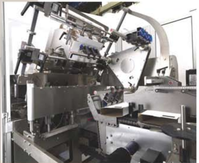
The Criterion 3 Cartoner from R.A. Jones, capable of reaching speeds of 330 cpm, features a three-head, servo-driven, rotary carton feed powered by a low-level carton magazine with an ergonomic 40-in. height.
