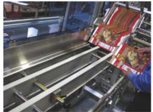
Low-level carton magazine improves ergonomics on cartoners from Langen Packaging.
