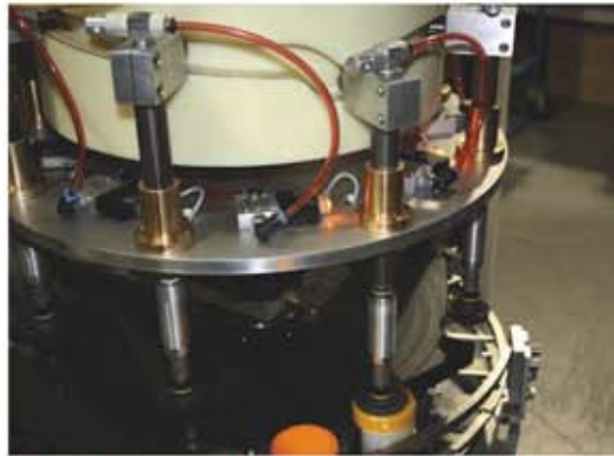
Compact rotary turret on servo-driven VC-VCA cartoner from AFA Systems replaces the traditional racetrack vertical loader. Design reduces machine size, moving parts and maintenance requirements and improves visibility into the machine.
