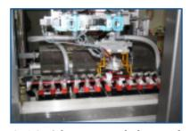
SUBO pick, group and place end effector allows the HD-LSP to effectively collate bulk product. This unit ensures a high quality pack pattern in the carton.
