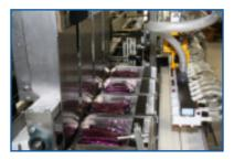
Innovative overhead confiners will complete the process of confining the product during loading and securing the product during accumulation
