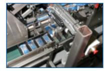
Servopack Infeed conveyor allows the HD-LSP to reach speeds of over 600 ppm. Dual servo driven belts allow the conveyor to simultaneously load and accumulate.
