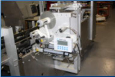
**AFA can retrofit its equipment to meet the customer's needs. In this application, AFA installed a labeling unit to combine two operations at one station.**
