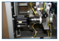
Servo motors on all major drives ensure smooth operation. In addition, feedback on fault diagnostic and positioning accuracy are accessible with the servo loader.
