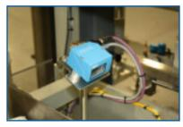
The CE-GRT's modular design allows retrofits and optional equipment to be integrated into the machine. Code daters, printers, bar code readers and more can be easily integrated.
