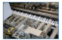
High-speed automatic barrel cam loader can meet your production speeds. A reverse barrel cam loader option is available for window style cartons and special cartons.
