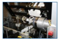
Rotary dual head feeder can achieve either continuous or intermittent motion carton feed. Furthermore, the feeder can accommodate a wide range of cartons.
