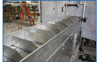
**Autoload Buckets allow for semi-automated cartoning. The buckets are adjustable and AFA will provide jigs for each SKU. This allows for accurate and repeatable changeovers.**
