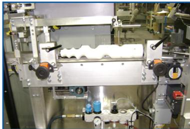
High speed bottle in-feed system with quick change timing screw coupling. This component reduces changeover time when switching carton and product sizes.
