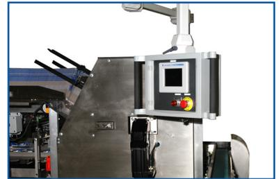
Swing arm operator panel offers an ergonomic solution for operators when troubleshooting machine faults. This feature also helps operators maintain the cartoner.
