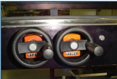
Digital scales allow operators to reference different carton and product configurations. This reduces changeover time resulting in better overall packaging efficiency.
