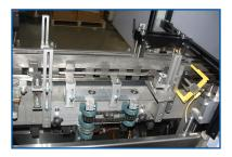
A variety of carton closing options are available including hot melt glue, tuck, lock tab, and auto bottom closing.
