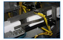
Detection systems are available to include on the MK-SML. Also, various bar code, open flap, and leaflet detection and rejection systems are available.
