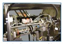
Optional reverse servo driven feeder with pre break vacuum cup can erect square cartons at a high efficiency rate and increase production speeds.
